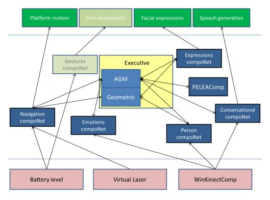
Fig. 1. Overview of the RoboCog architecture. Green upper blocks are low-level action components, pink low blocks are low-level perception components and blue blocks are networks of componets unfolding a specific functionality. The yellow block is the Executive center that sequentiates the activity and routes traffic among the blocks. Blurred blocks show modules not integrated in the specific instance of the architecture described in this paper.
